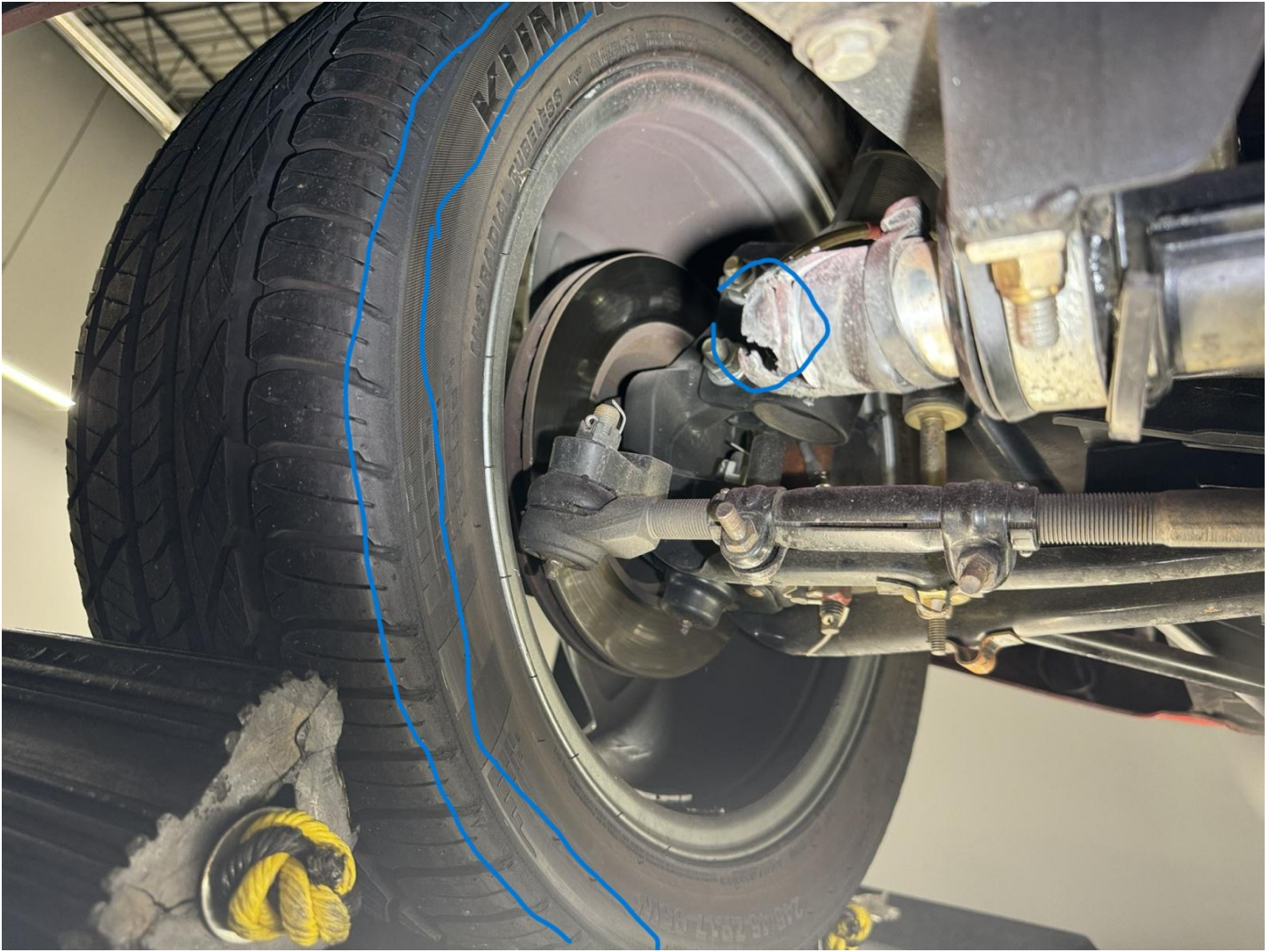
left tire touches the steering rack
