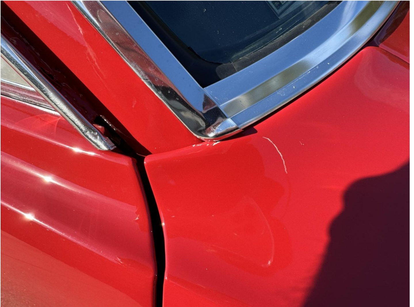
Body damage: Right quarter panel
