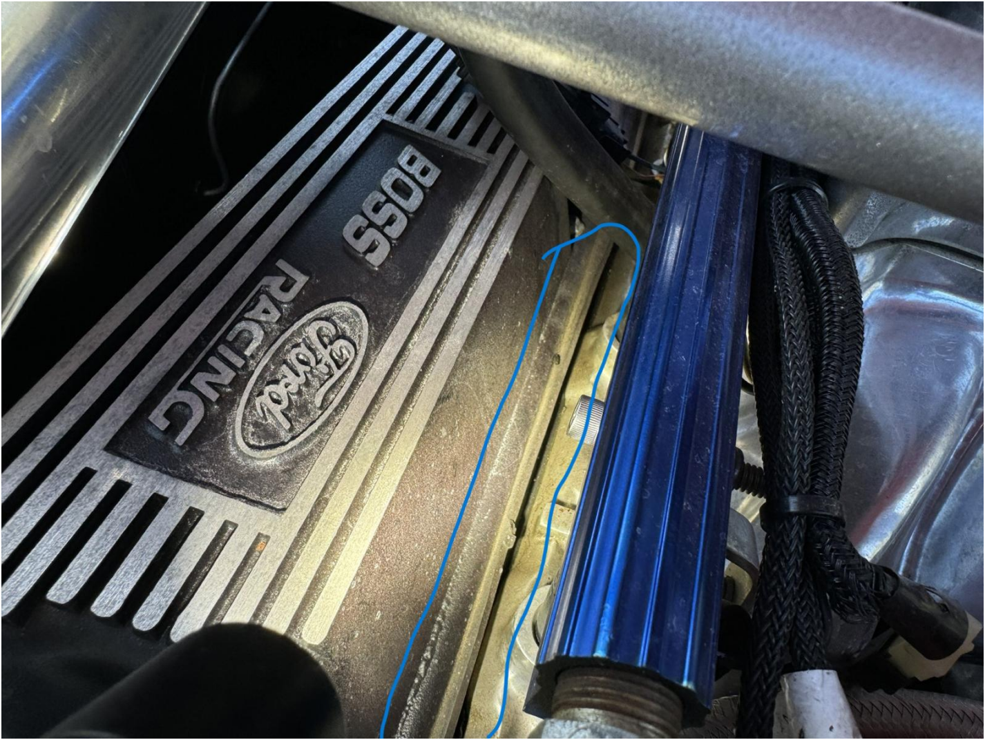
valve cover oil leak
