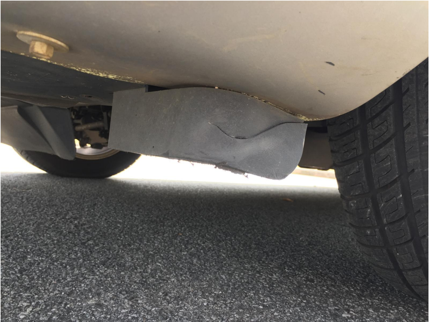
cracked air deflector
