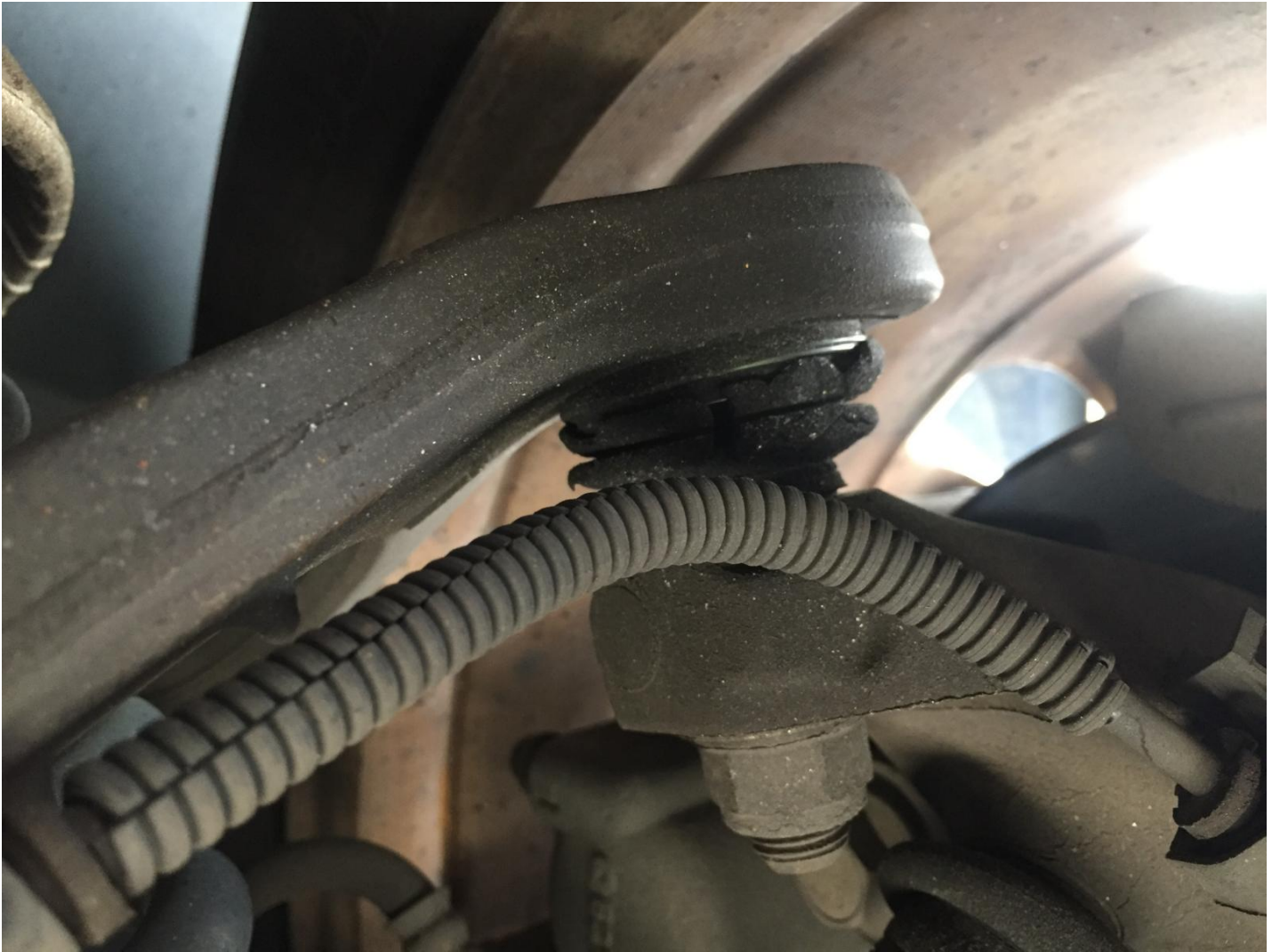
Left front upper ball joint. Torn boot.
