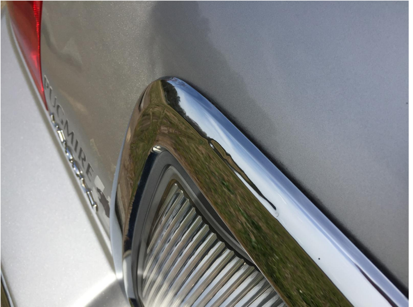
chrome trim peeling
